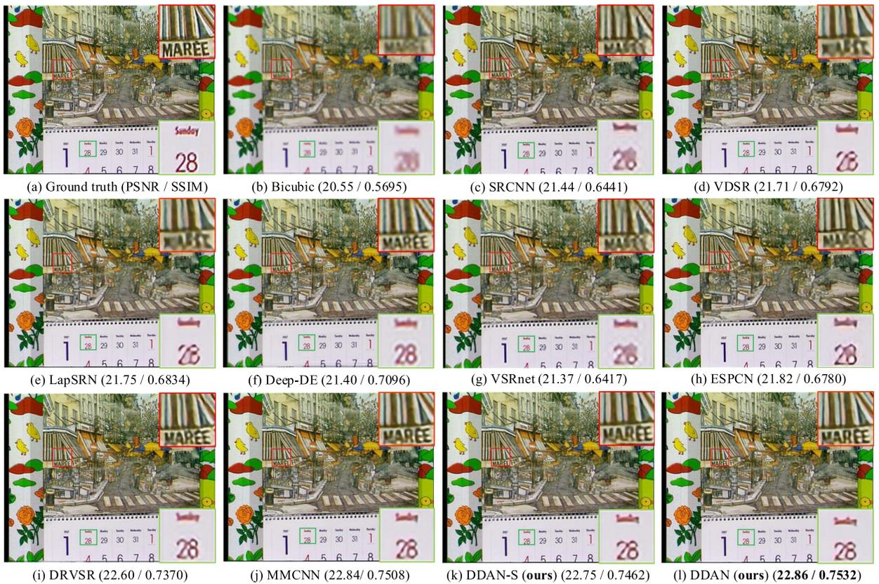
Fig. 11. Visual comparisons on the 15<sup>th</sup> frame from *calendar* for 4 $\times$  SR.
